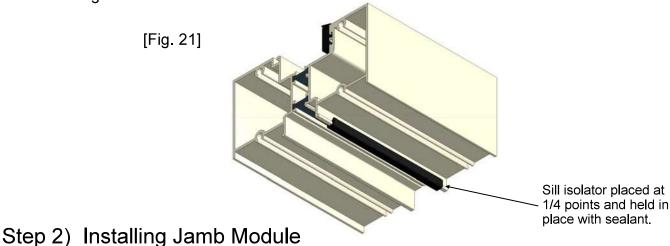
Place the module on the subsill at an approximate 30° angle. While applying pressure upward, rotate the module into the condition. See figure 22. When rotated correctly into place, the interlocking legs of the sill will set inside the lock cavity of the subsill; the sill should set flat on the subsill. See figure 23 for sill placement on the subsill.
