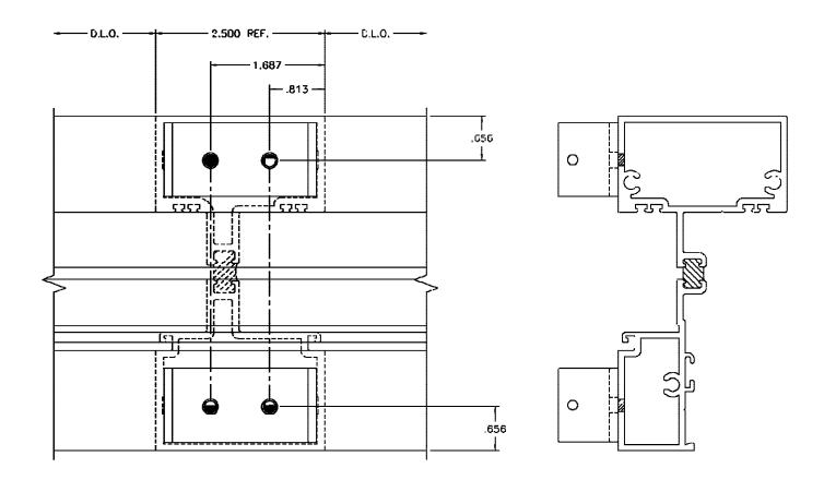
This fabrication works with vertical attaching to either the head, horizontal, or sill.
