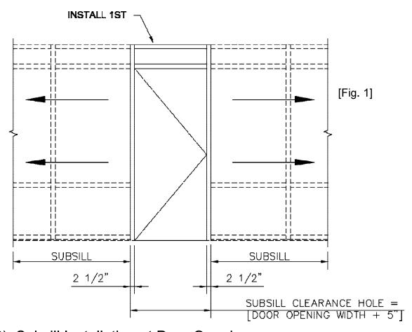
Step 2) Subsill Installation at Door Opening
