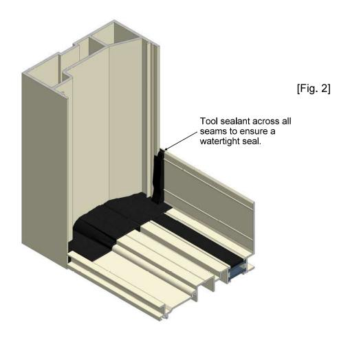
NOTE: Fill the glazing pocket of the door jamb flush with the sealant to the tallest portion of the subsill that bridges the pocket. Tool the silicone so a watertight seal is made to make sure that water will be directed out of the glazing pocket and into the subsill.
