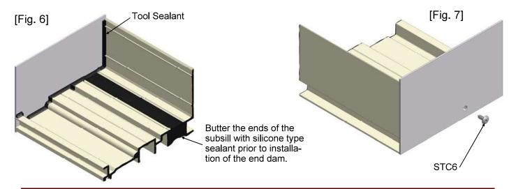
Prior to applying sealant to the required areas, clean the area with Isopropyl Alcohol and a clean towel that will not leave towel materials behind. Wipe off material with a sufficiently dampened towel to remove all dust, oil, and cutting fluids from the required areas. Allow to air dry before applying any sealant.
