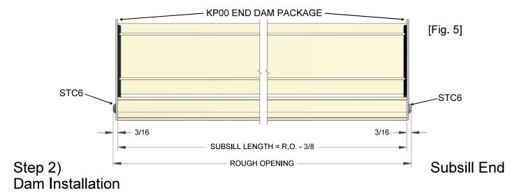
Prior to installing the end dam, apply a generous amount of silicone type sealant to the end of the subsill. Insert the STC6 fasteners into the end dam, and attach it to the end of the subsill. After the end dam is attached, the excess sealant should be tooled at the interior of the subsill/end dam joint to provide a watertight seal. Apply more sealant, if required, for a watertight seal. (See figures 6 and 7.)
